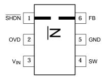
Note: This IC could be destroyed in some case if amounted in 180° inverse direction. Please be careful about IC direction in mounting.
