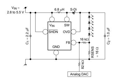
4) Input PWM signal with filtering to FB terminal
